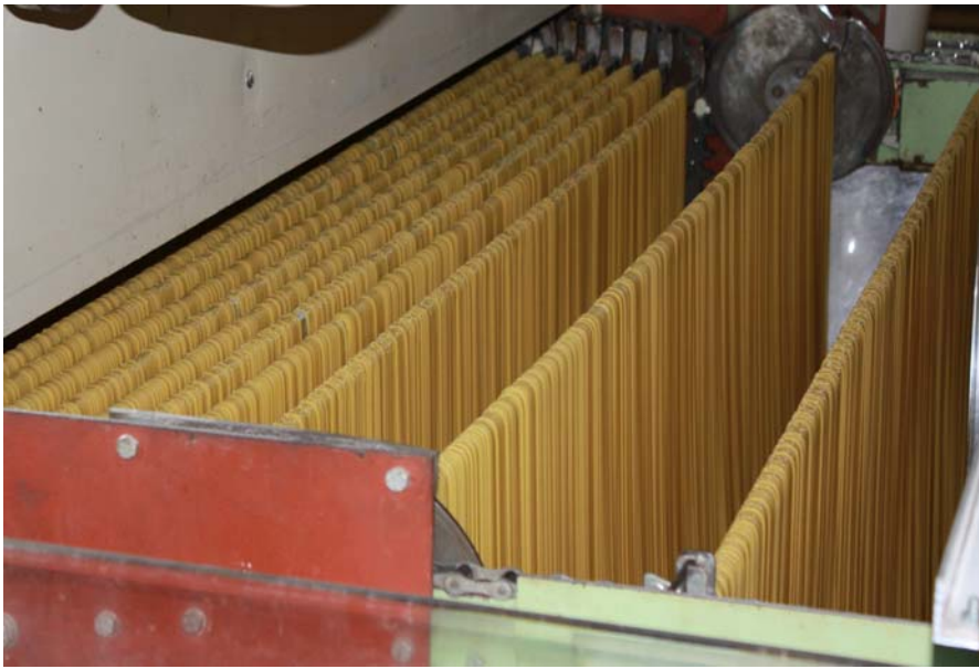
Figure 3 - Spaghetti hangs on bars as it enters the dryer
