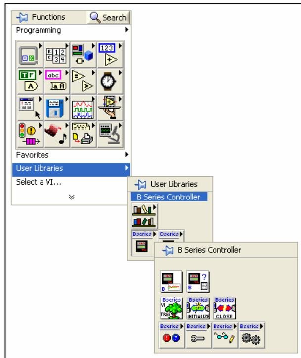
Figure 1 - B series Controller VIs under User Libraries on the Tools Palette
