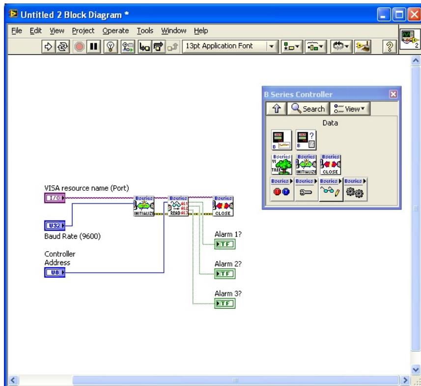
Figure 5 – Basic Application VI block diagram
