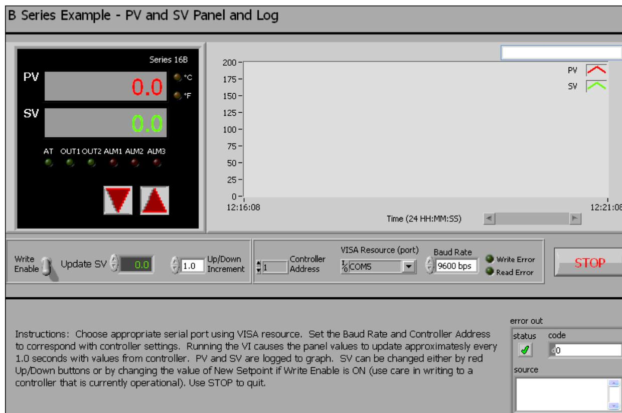
Figure 3 - B series Example - PV and SV Panel and Log.vi front panel
