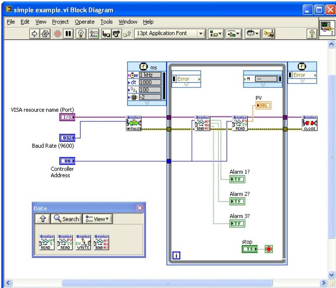
Figure 6 - Simple Example VI block diagram
